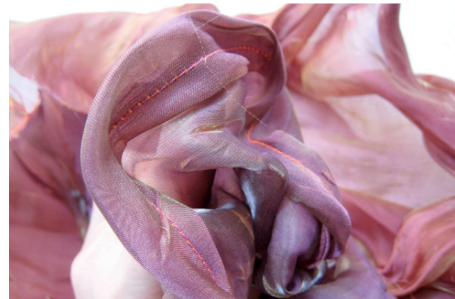
figure 1. This wired apparel alerts the user by mechanically shrinking the fabric onto specific points of tensions on the body.
